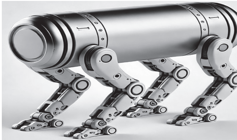
FIGURE 1.3 Quadrupedal robot. The dog-like robot weighs 9 kg and has 12 actuated joints (three per leg), making it well suited for dynamic locomotion research. It measures approximately 24 cm in height and 40 cm in length. The figure is reproduced from reference [10].
